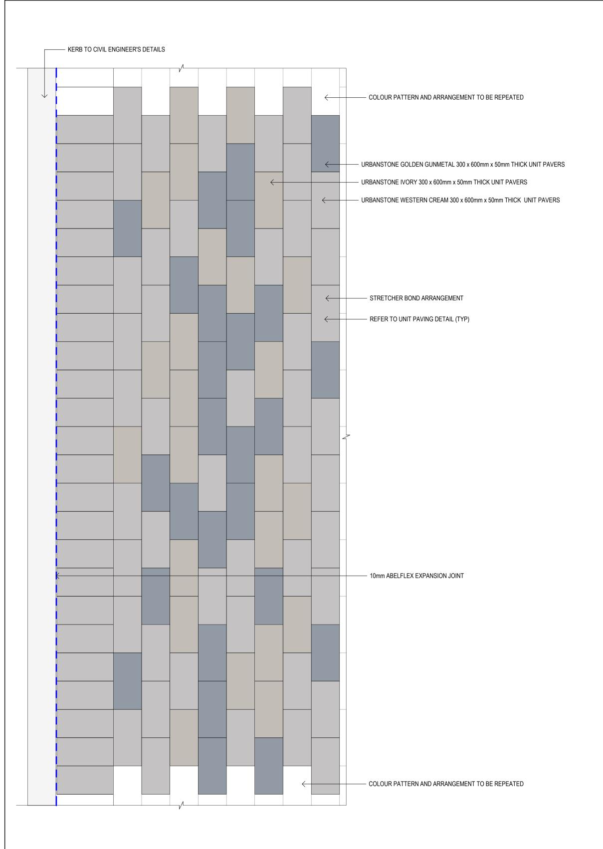
UNIT PAVING TO BE ARRANGED IN STRETCHER BOND ARRANGEMENT AND COLOUR PATTERN TO BE SIMILAR AS PROJECT EXAMPLE ON THE RIGHT IMAGE
